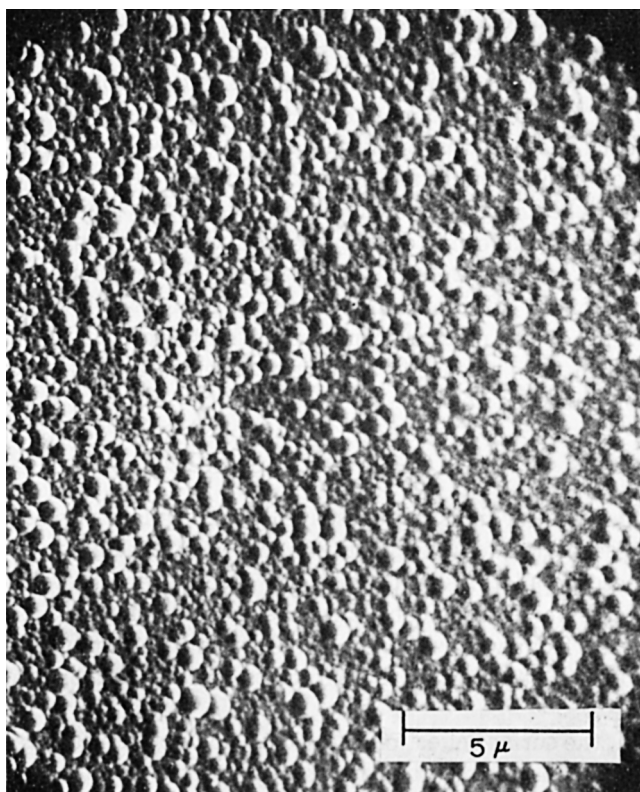
Fig. 1. HMDS polymer film deposited on aluminum.
